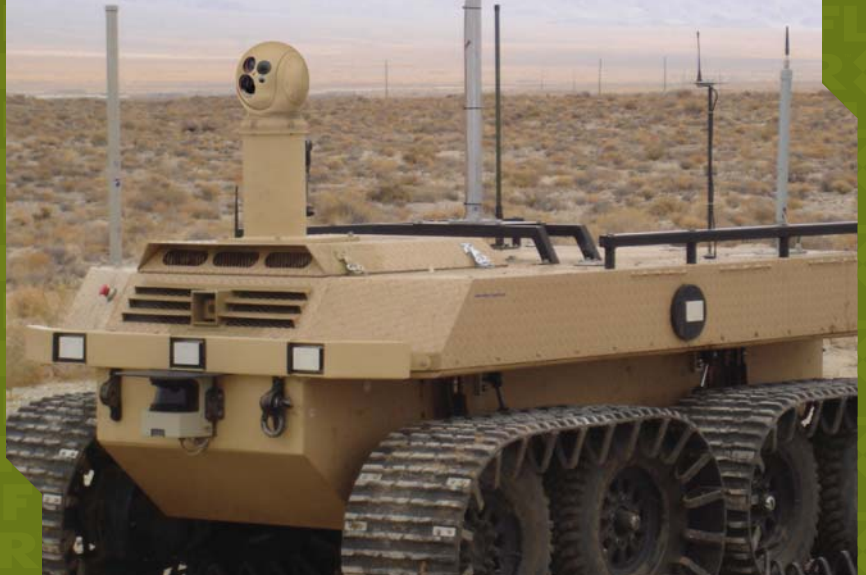
TacFLIR system on the Remotec TAGGS Unmanned Land Vehicle
